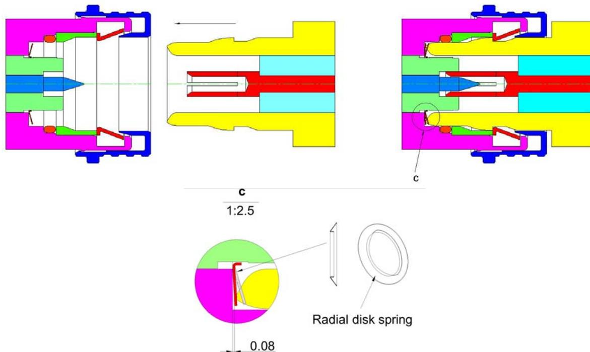
Fig.3 QLF'S QN (2004) with radial disk spring
