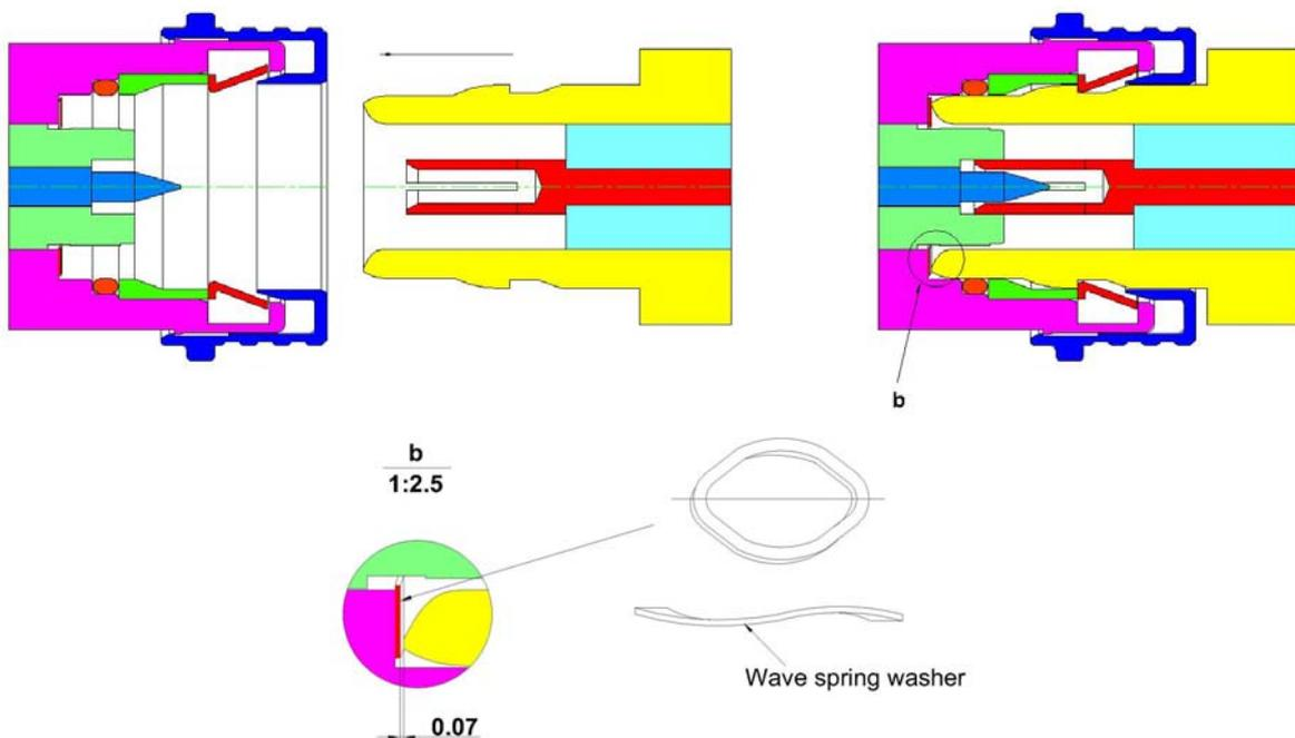
Fig.2 QLF'S QN (2003) with wave spring washer
